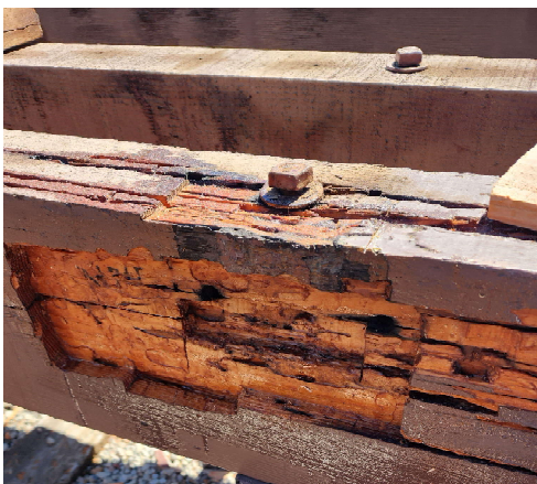
From left to right: John Stutz, Hanson Loey, and Tony Peters hard at work on picnic car 1725. Notice all of the dark spots on top of the sills... the crew is working on cleaning and treating termite damage in every location.
