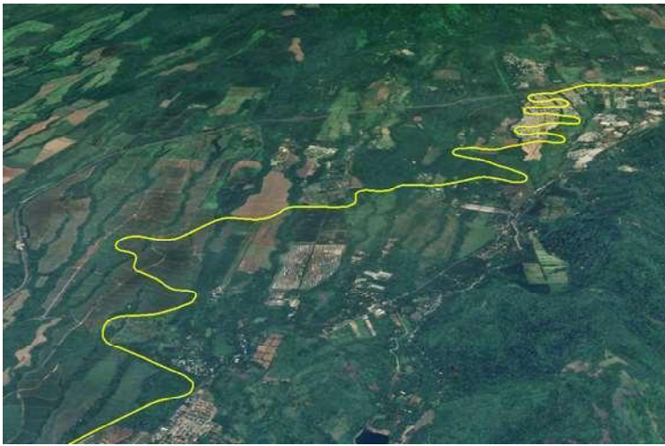
Guatemala Central turn-backs near Escuintla. This section was originally a 4.5% grade rebuilt to 3.5% in 1889.
