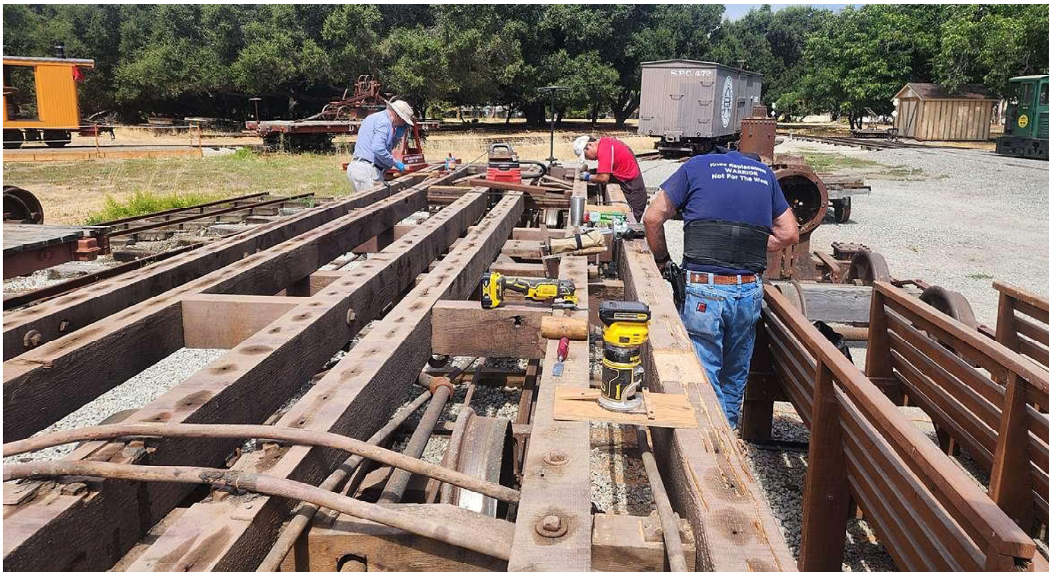
From left to right: John Stutz, Hanson Loey, and Tony Peters hard at work on picnic car 1725. Notice all of the dark spots on top of the sills... the crew is working on cleaning and treating termite damage in every location.
