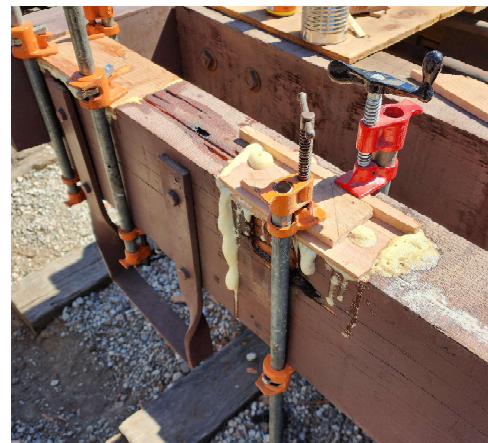
From left to right: John Stutz, Hanson Loey, and Tony Peters hard at work on picnic car 1725. Notice all of the dark spots on top of the sills... the crew is working on cleaning and treating termite damage in every location.
