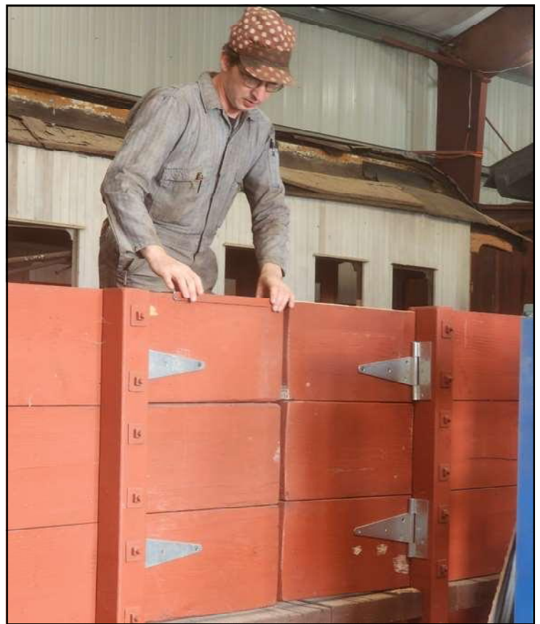
David Waterman fitting the new doors onto WSL Co. 222.
