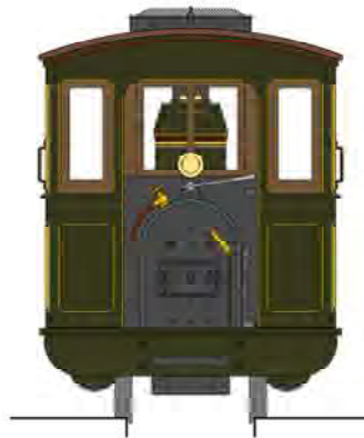
R.E. WOODWARD, MOOR'S STATON, BUTTE Co. CAL. 'CHAS. KOHLER' BALDWIN LOCOMOTIVE WORKS CLASS 6-10D2, DRAWING 2 CONSTRUCTION No 7362, 1884 36" GAUGE PAINTING STYLE - OLIVE GREEN & COLOR, STYLE 133 LOCOMOTIVE PRESERVED IN PARTS AT THE RAILROAD MUSEUM AT ARDENWOOD, CA
