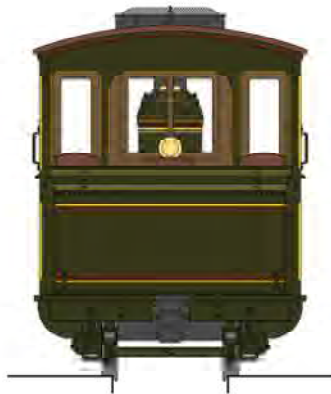
R.E. WOODWARD, MOOR'S STATON, BUTTE Co. CAL. 'CHAS. KOHLER' BALDWIN LOCOMOTIVE WORKS CLASS 6-10D2, DRAWING 2 CONSTRUCTION No 7362, 1884 36" GAUGE PAINTING STYLE - OLIVE GREEN & COLOR, STYLE 133 LOCOMOTIVE PRESERVED IN PARTS AT THE RAILROAD MUSEUM AT ARDENWOOD, CA
