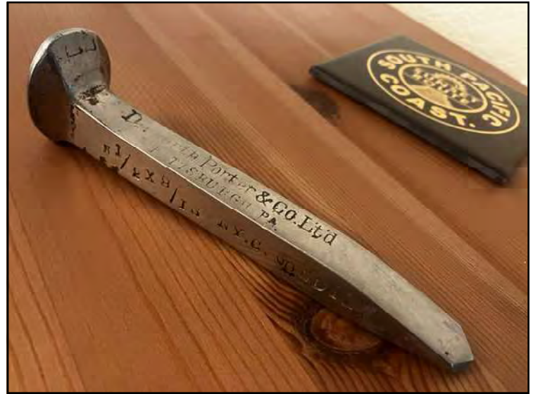
Dilworth Porter & Co. Ltd was located in Pittsburg, PA and produced "Goldie" spikes. This polished sample (note the chisel tip) is engraved with the company name, and also 5 1/2 x 9/16 N.Y.C. GOLDIE.
