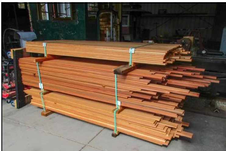
The milled old growth redwood is sandwiched in between the Douglas Fir to protect it. Photo by Don Marenzi
