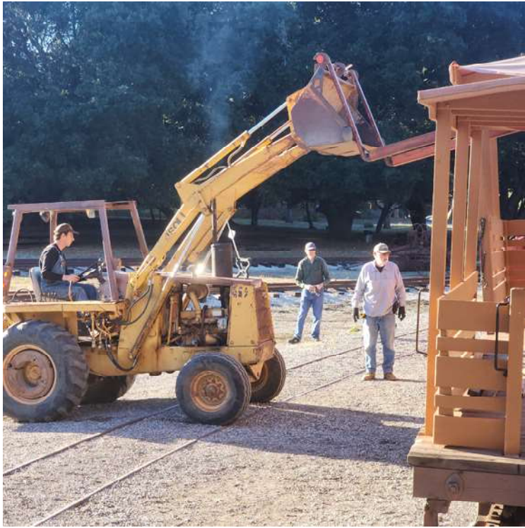
After three decades of service NS flat car 1725 needs some necessary repairs. Here David Waterman is moving the tractor forks into position to lift the roof off as Tom Sturm and Tony Peters watch.
