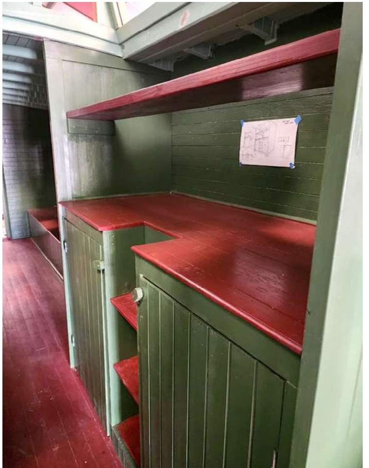
The inside of NWP caboose 6101. This photo shows the cabinetry and steps for the cupola seats (not installed yet). Beyond is the bench seats.
